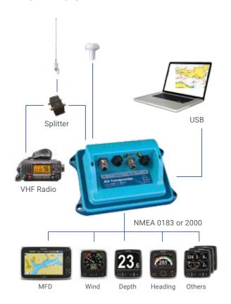
The only AIS transponder with fast 5Hz GPS navigation rate. Use the XB-6000 as your primary GPS source for your NMEA 2000 and NMEA 0183 equipment.
