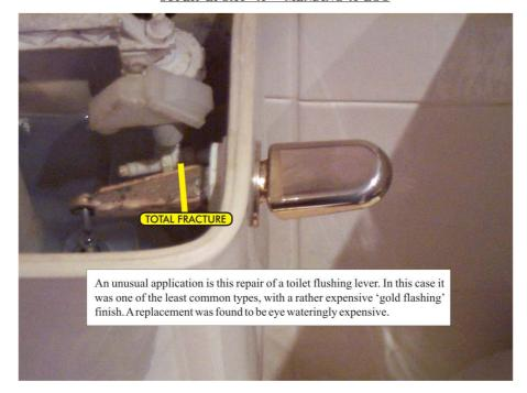
The lever was a nylon moulding, a material not given to bonding well with any epoxy system, so it was decided to try a 'secondary structure' using a cut down steel screw to mend the lever. The metal on its own would provide some strength but its main purpose was to hold the two pieces together whilst the wooden spatulas, with the mix of Blue Gee Epoxy 'A' and Microfibres set. The repair is still OK after 12 months use.
