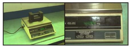
The left hand picture shows the instrument after it had been Epoxy 'A' over coated using 165g/Sq.M. Glassfibre Tape as a reinforcing substrate. Note the clarity of the display shown in the right hand picture *(cleaned with acetone!)* - after many years use.
