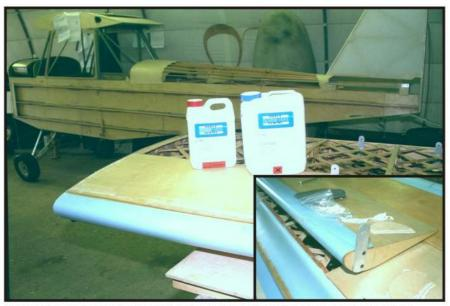
The inset shows the details of wing trailing edge, together with an aileron in course of construction.
